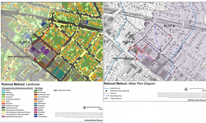
Figure 1: Rational Method Landcover (left), Waterflow (right) diagram. (Source: Author.)
