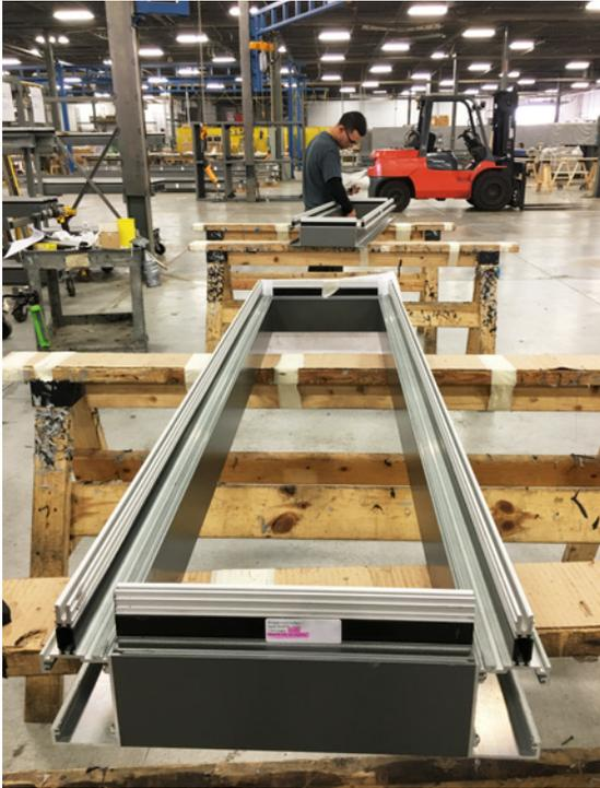
Figure 6: Thermally broken aluminum frame.
