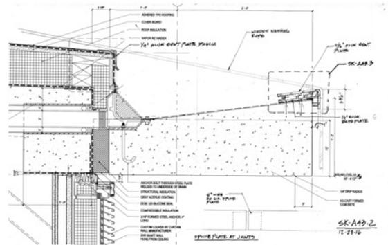
Figure 10: Section through soffit.
