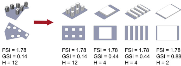
Figure 6: FSI and GSI comparison of the TOKI Etiler project with different building patterns.
